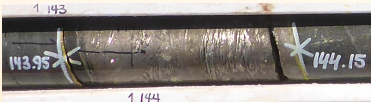
Figure 4 – Close up core photo of massive sulphide intercept in DMDD0003 at Conductor C. Interval (0.2m downhole) assayed 6.35% Ni. Note core is HQ3, with a diameter of ~61.1mm.
