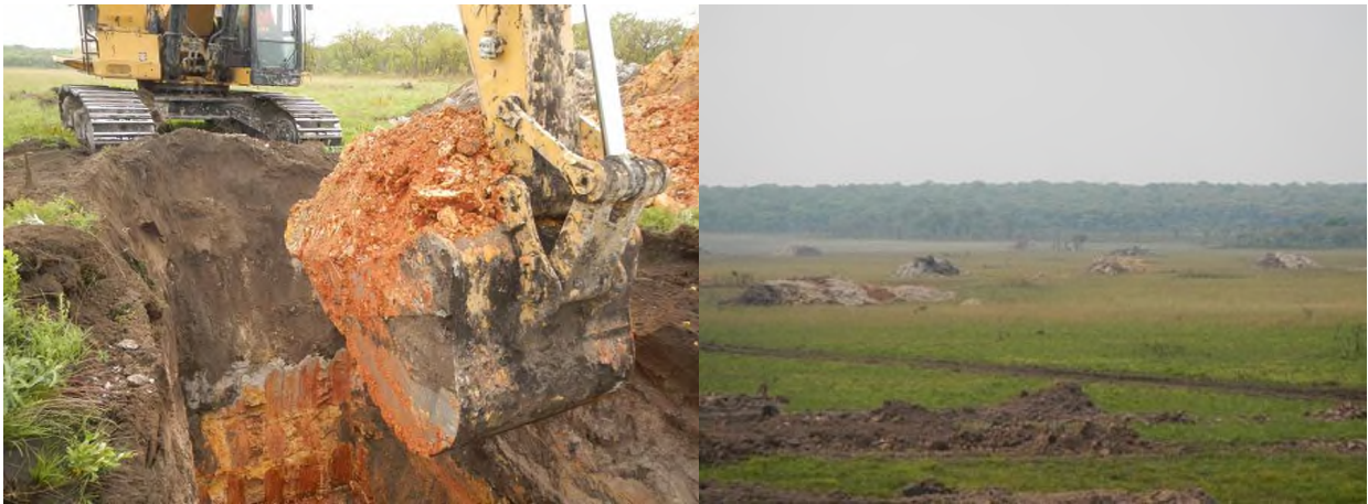
Figure 2: Excavator pitting over the kimberlite target area
