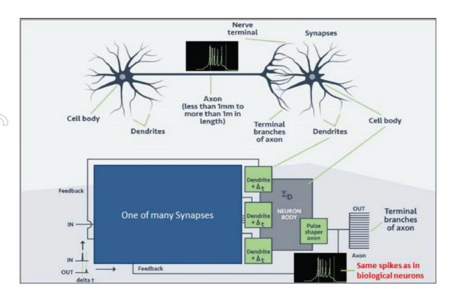
Each artificial neuron in BrainChip's SNAP technology is a separate circuit that works in parallel (all at once), as set out in the diagram below:
