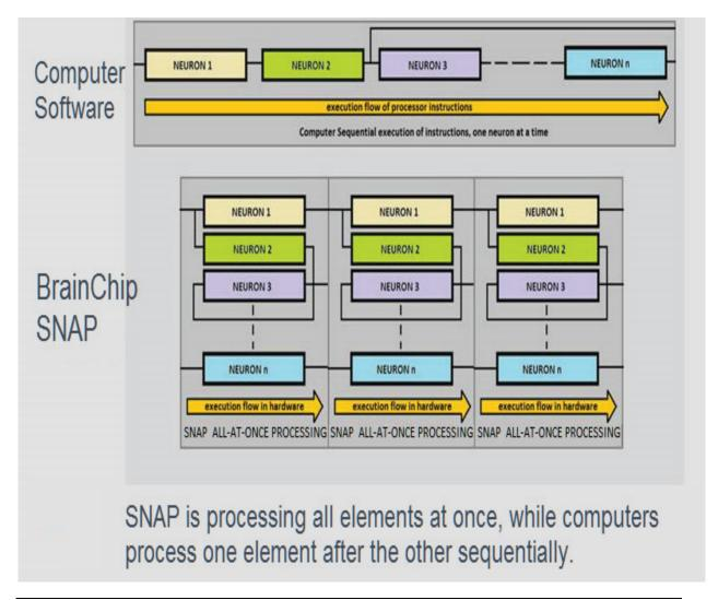
Each neuron in the BrainChip SNAP technology is updated in parallel, resulting in faster processing times compared to current software ANNs. This is a significant difference, because software ANNs slow down when they get larger due to their sequential processing method. The larger the neural network is, the greater the speed advantage of the BrainChip SNAP technology is.
