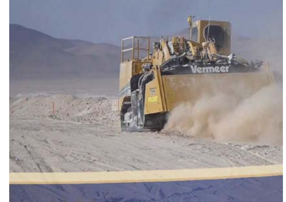
Salt extraction using surface miners
