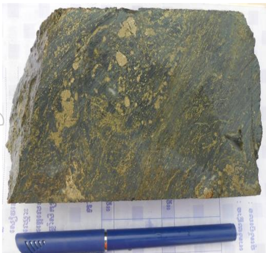
Image 1: Prospect 128 hole KDH075- Copper mineralisation at 37.40-37.55m
