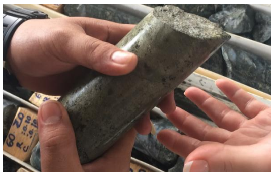
Image 2: Massive Chalcopyrite from Prospect 128
