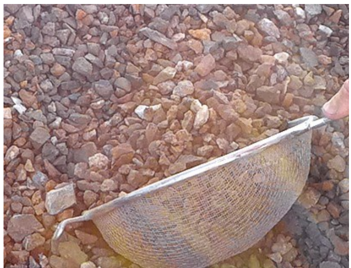
Figure 6: Crushed ore stockpiles (-40mm) grades are estimated from a combination of lab-assay of composite blast-hole samples and where not available, resource grade estimates are used. Check assays are regularly conducted for QAQC purposes.
