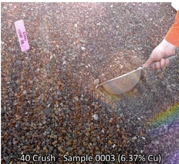
Figure 6: Crushed ore stockpiles (-40mm) grades are estimated from a combination of lab-assay of composite blast-hole samples and where not available, resource grade estimates are used. Check assays are regularly conducted for QAQC purposes.
