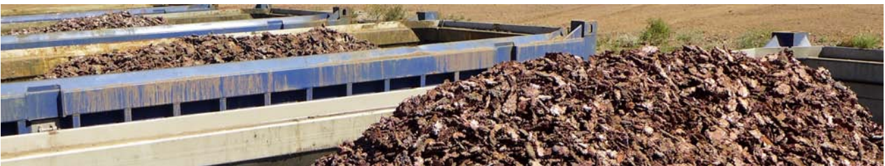
Figure 2: Oversize native copper metal concentrate ~95% Cu loaded into containers at Rocklands prior to shipment to Townsville.
