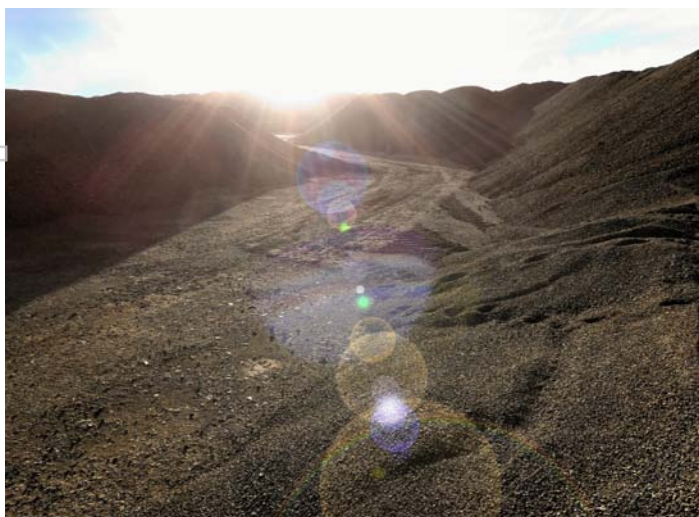
Figure 7: Crushed ore stockpiles (-40mm) grades are estimated from a combination of lab-assay of composite blast-hole samples and where not available, resource grade estimates are used. Check assays are regularly conducted for QAQC purposes.
