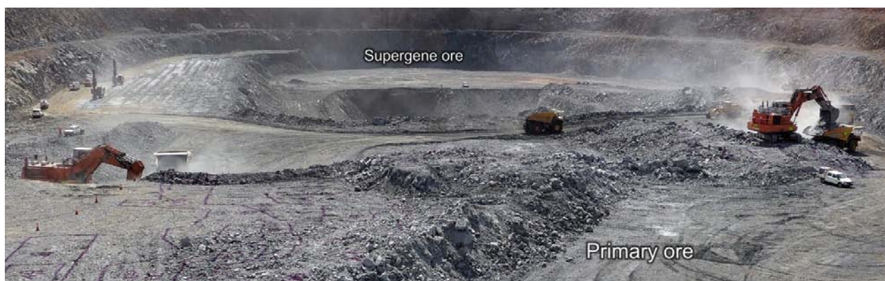
Figure 12: Concurrent mining of supergene ore in the north and primary sulphide ore in the south of the LM2 Pit at RL190 - ore mark-up can be seen on pit floor.
