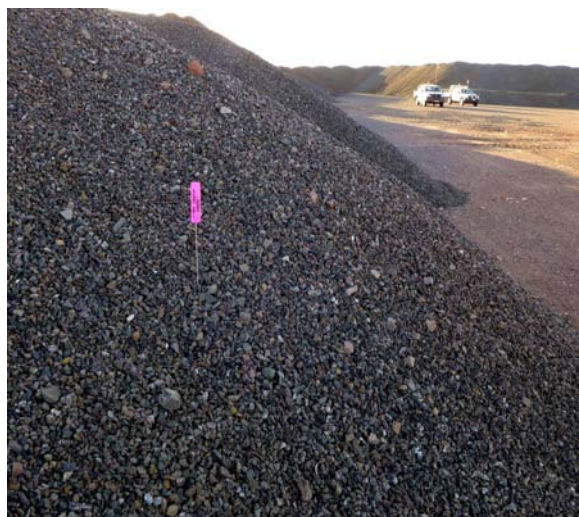
Figure 7: Crushed ore stockpiles (-40mm) grades are estimated from a combination of lab-assay of composite blast-hole samples and where not available, resource grade estimates are used. Check assays are regularly conducted for QAQC purposes.
