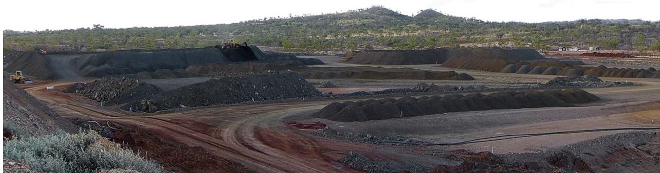
Figure 5: Crushed ore stockpiles (-40mm) will be fed directly into the Process Plant without further crushing, and are currently over 200,000 tonnes.
