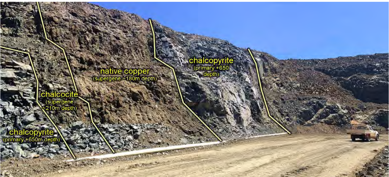
Figure 11: LM1 Pit wall above south haul-road (~45m below surface), showing sub-parallel ore zones that include primary sulphide ore types (chalcopyrite & bornite) and supergene ore types (chalcocite & native copper) in vertically stacked, sub-parallel zones.
