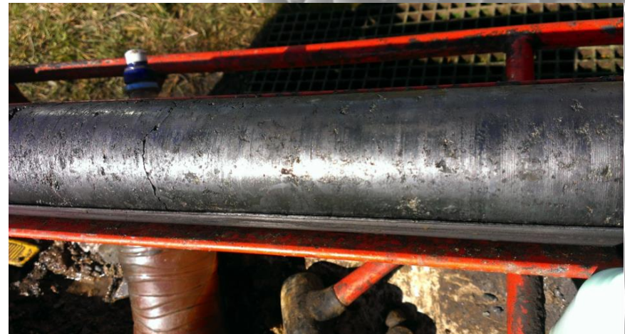
Core sample from new pegmatite zone
