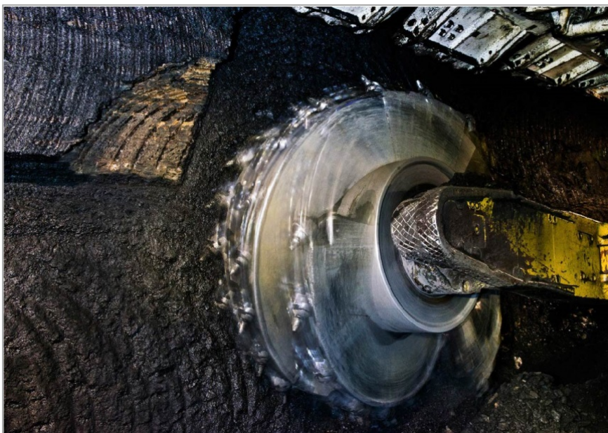
Figure 4: Typical Longwall Shearer
