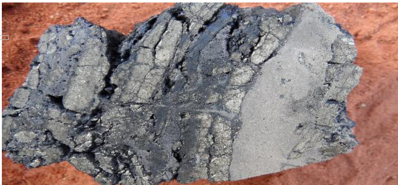
Mineralised horizon with replacement pyrite and chalcocite from diamond drillhole EUR14DD009
