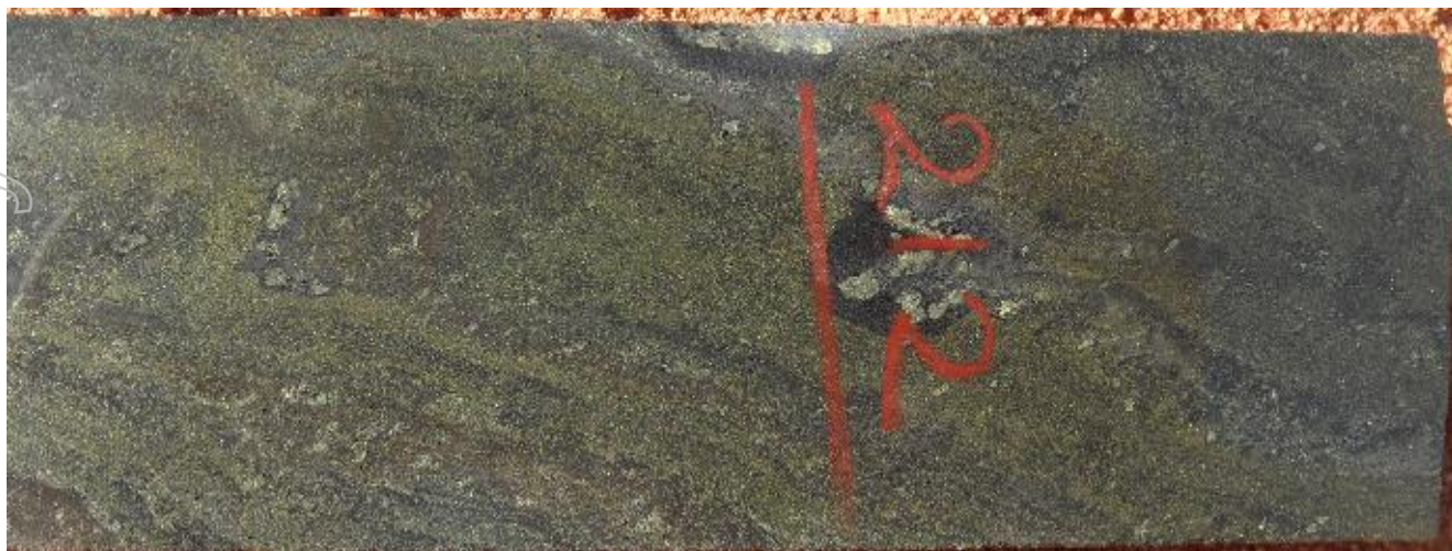
MMG diamond drillhole BRK14DD001A from 212m depth showing laminated chalcopyrite (copper sulphide-brassy yellow colour) and dark grey magnetite replacement bands. This interval carries more than 2% copper.
