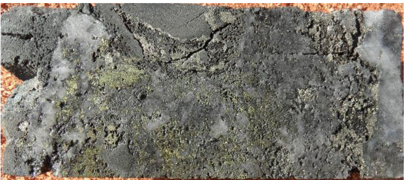
Detail of portion of downhole interval containing 6m @ 5.3% Cu from 157m in diamond drillhole EUR14DD009 from Eurinilla Dome.
