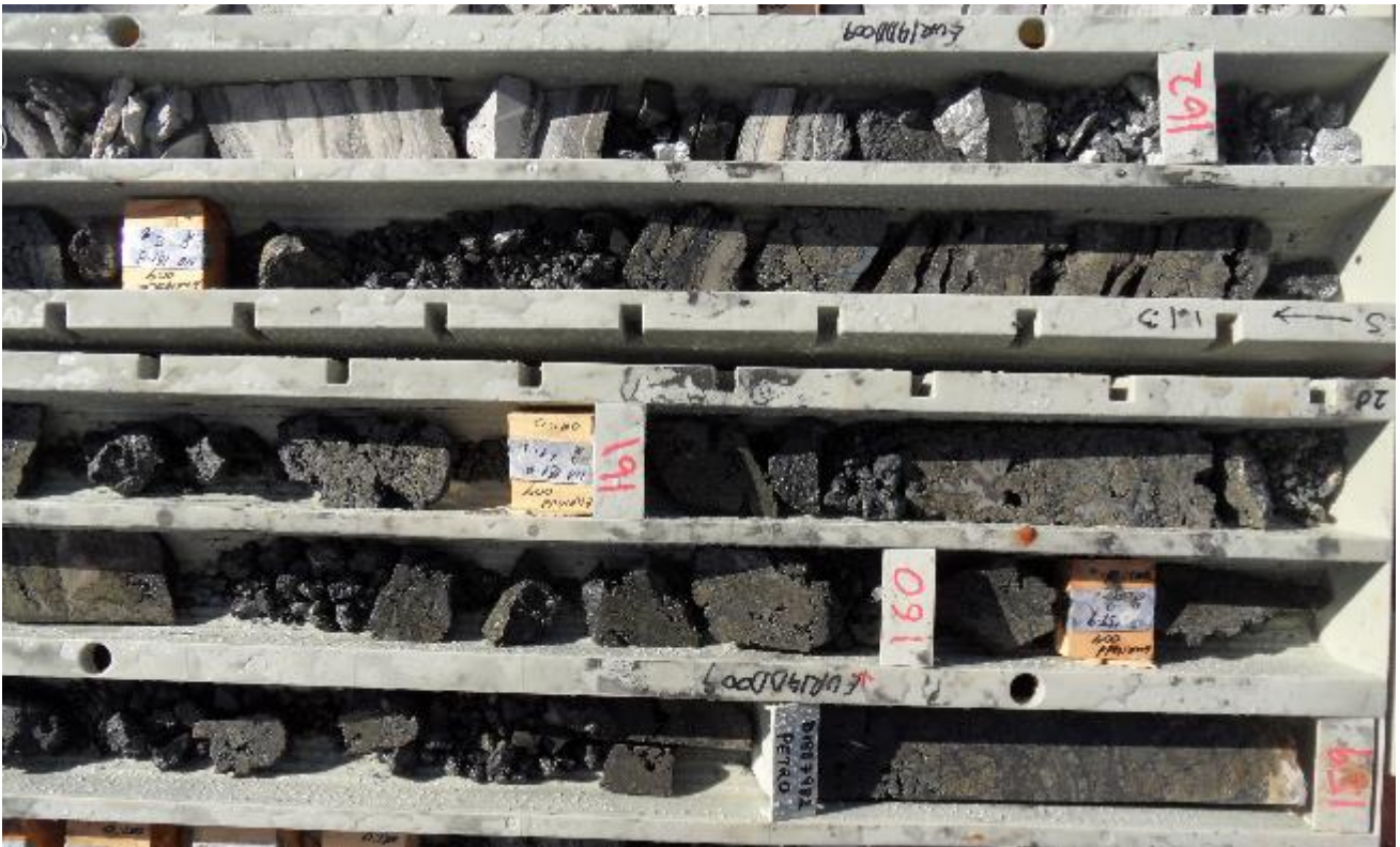
Portion of downhole interval containing 6m @ 5.3% Cu from 157m in diamond drillhole EUR14DD009 from Eurinilla Dome. This is replacement mineralisation occurs within a portion of the so called "mineralised horizon" that runs for more than 200km through Havilah's tenements and is host to the Kalkaroo and North Portia copper-gold deposits.
