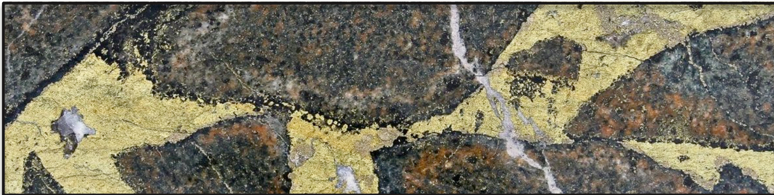
KHDDH346: 415.5m. From a 2m interval (414m to 416m) that assayed 5.16% Cu & 3.44 g/t Au
