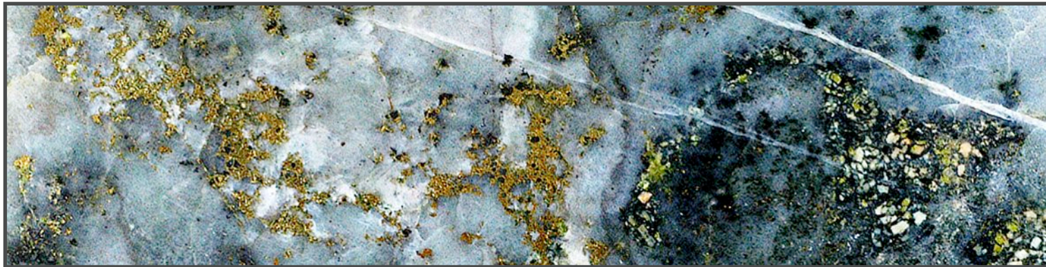
Massive granular quartz-chalcopyrite-magnetite vein: 2 metres @ 6.25 g/t Au and 2.52% Cu
