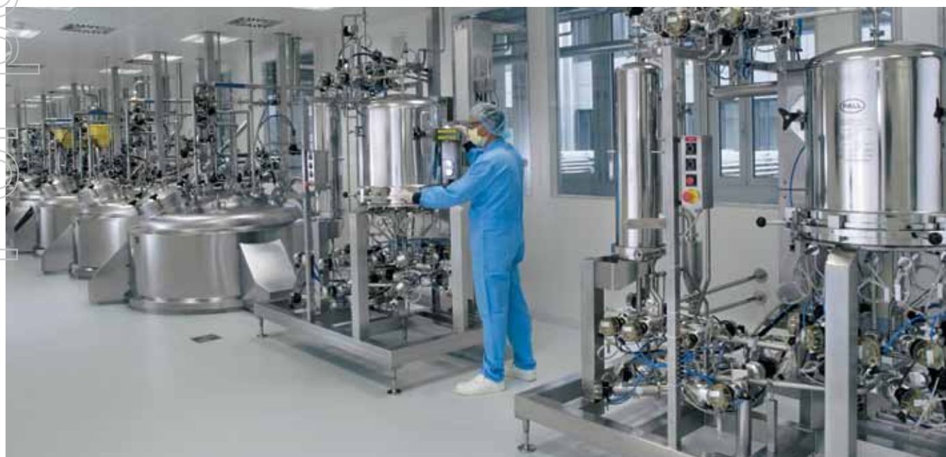
Inside the IgLAB bulk manufacturing facility in Bern where chromatography and virus filtration operations are carried out for Privigen® and Hizentra®.
