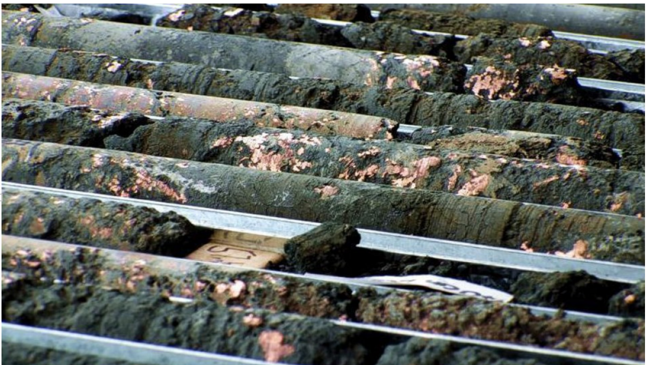
Figure 8: Diamond drill hole LMDH007 - among the first few diamond holes drilled into Las Minerale in the early days of the discovery. Above; copper filings can be seen remaining in the water-return wash-back (above) and drill core from the Bonanza area (intersected in LMDH007) about to be accessed in the pit (~51m +/- 5m)
