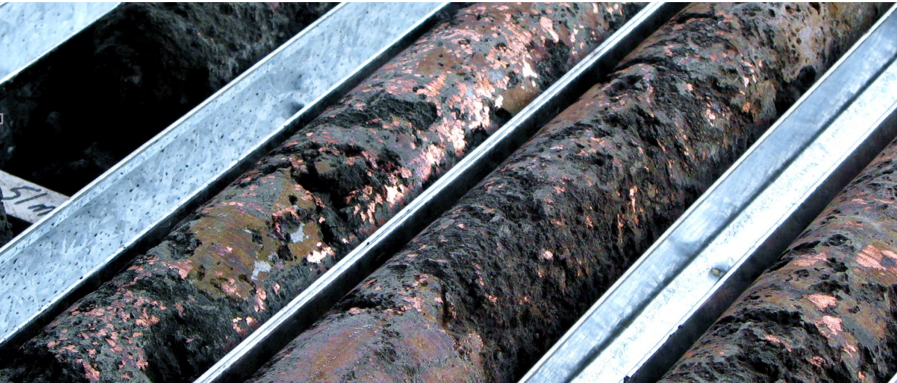
Figure 7: Examples of coarse native copper in metallurgical drilling in the Bonanza native copper ore zone.
