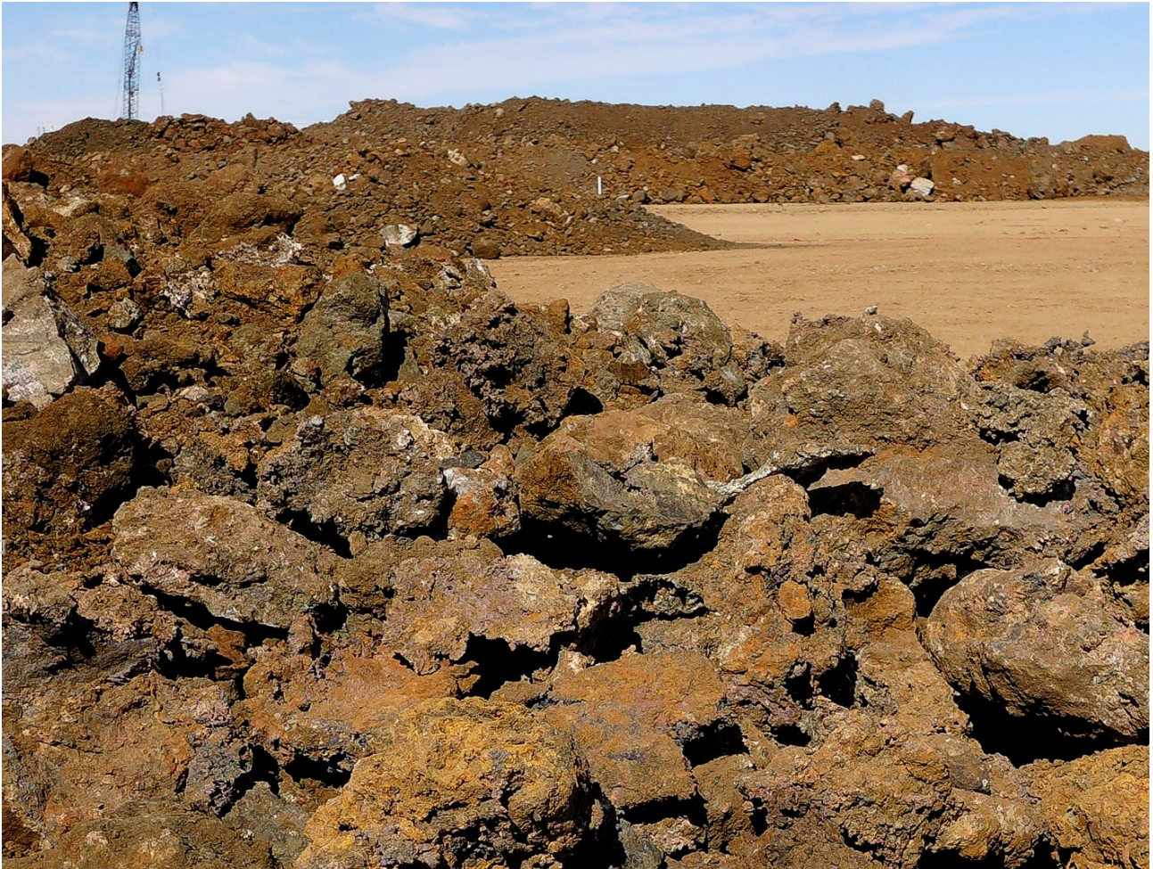
Figure 1: Large, (up to 4 tonne) coarse native copper masses building on the various ROM DSO stockpiles (native copper contains 99.65% copper metal). Crushing circuit being modified to screen and process larger than expected masses of native copper for DSO.
