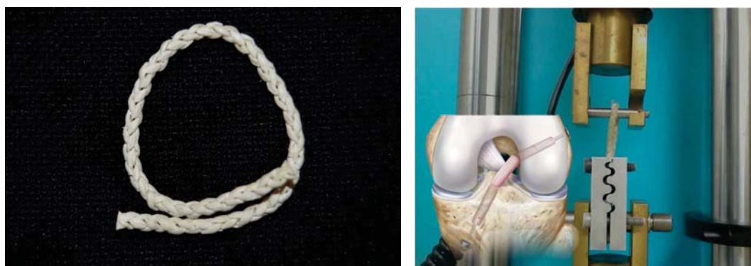
Figure 12 - CelGro™ collagen tendon and biomechanical testing (600N/ 4mm cross-section)
