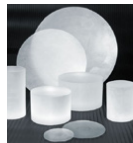
Artificial sapphire made from >4N Al 2 O 3
