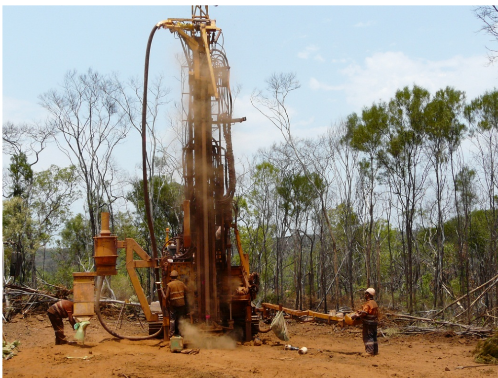
Mountain Creek project - Reverse Circulation drill rig.
