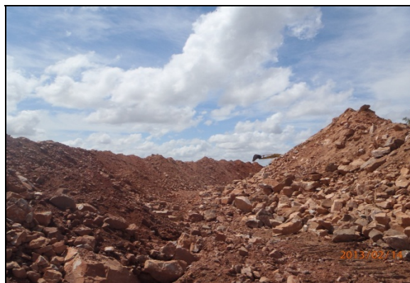
Stockpiled crusher feed material for concrete aggregate
