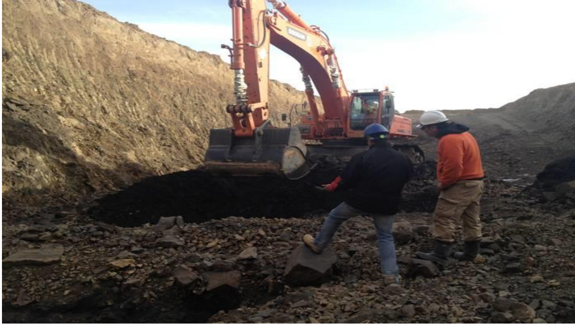
This photograph shows Geologists supervising an excavator on the floor of the test pit that is starting to dig into a coal seam for the purpose of taking samples.
