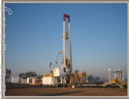
Coil-tubing drill rig
