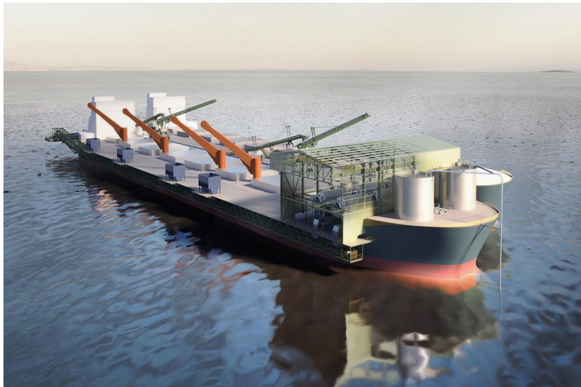
Figure 2: The Dewatering Transshipment Vessel (DTSV) configuration. Slurry is delivered directly to the surge tanks shown on the bow and dewatered by pressure filters (aft of the tanks). Dried concentrate is stored in the DTSV's holds for transfer by automated clam bucket cranes to the ocean going vessel shown behind the DTSV.
