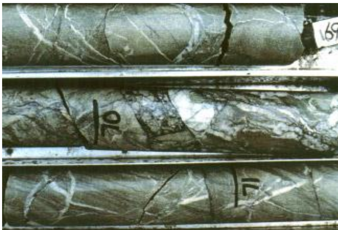
Plate 1. Photograph of drill core from MDD-001. Typical chalcedony-comb quartz vein stockwork mineralised zones in sericite altered thinly bedded sandstone at the Gettysberg prospect. Note the black chlorite-graphite-pyrite stylolite margins to chalcedony-comb quartz vein breccia. (Assay 70-71m: 0.37 ppm Au).
