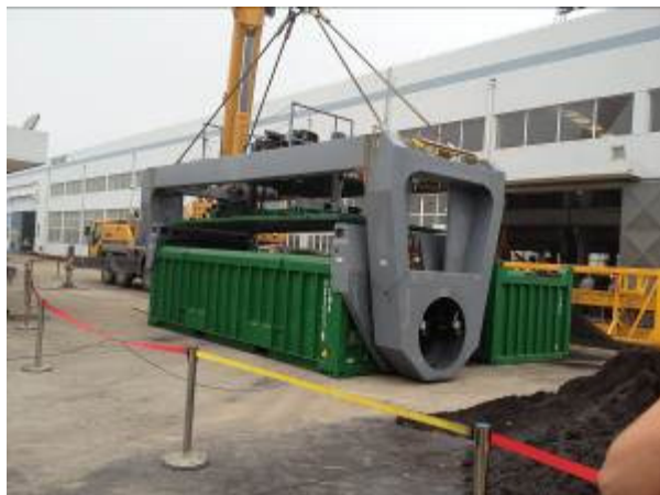
Figure 4: Rotating Spreader acceptance testing in China
