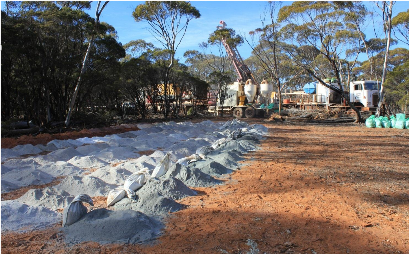
Figure 1. Discovery hole SFRC0024, Saturday 21 st July 2012. Note the run of darker grey samples (with disseminated sulphide) culminating in the black samples (matrix to massive sulphide).
