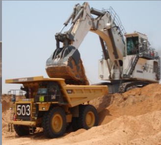
Liebherr 9350 Excavator and Caterpillar dump truck
