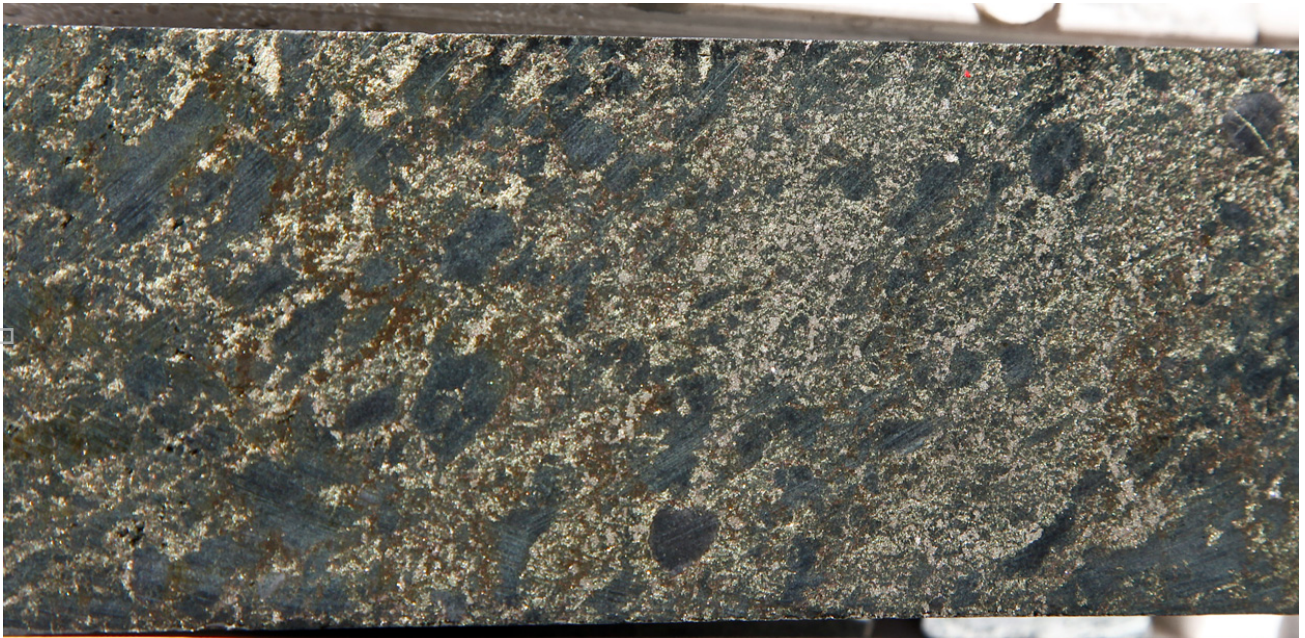
Photo 1 : A Zone Prospect. Chalcopyrite and pyrrhotite in lapilli tuff rocks from drill hole YRC11 - 41D approximately 280 metres down hole. Core approximately 5 cm wide.
