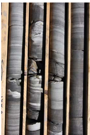
Figure 2-14: Marginal Paralic Sequence Uncovered in BTE-005
