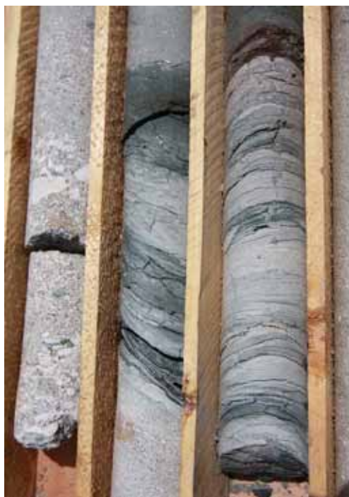
Figure 2-12: Lower Delta Plain Sequence from Drill Hole BTE-003
