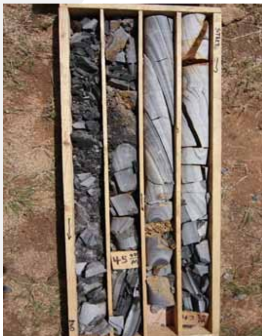
Figure 2-13: Steeply Dipping Proximal Overbank Deposits (BTE-004)
