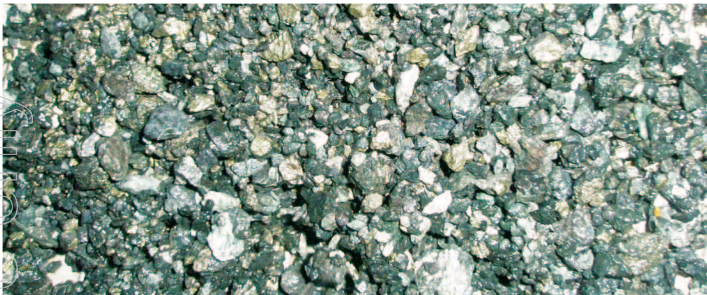
Figure 6-8: Washed chip sample from the richer copper intersection in SG1 at Silver Valley (the larger chips are up 2 cm across).
