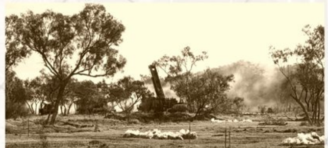
RC drill rig and sample bags
