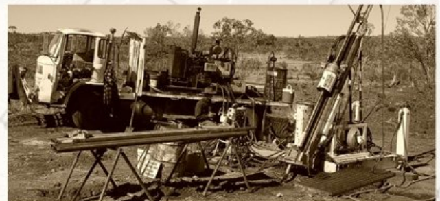
Diamond drill rig
