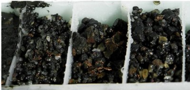
Native copper in drill chips
