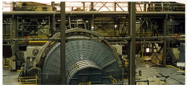
Typical large scale SAG Mill
