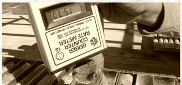
Geiger counter readings over Pitchblende in Wilgar core
