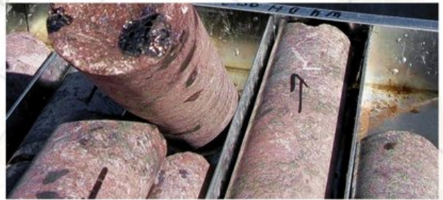
Diamond drill core...pitchblende (uraninite)
