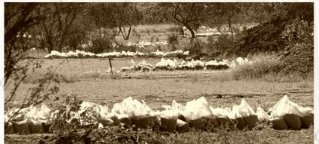
RC drill chips bagged and waiting
