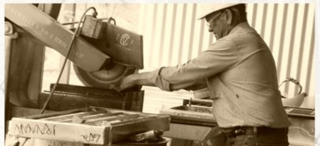
Diamond core splitting prior to dispatch to SGS labs
