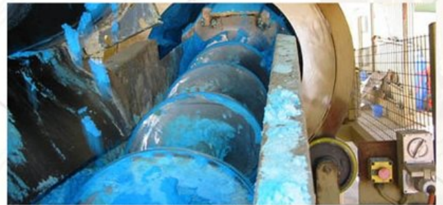
Copper sulphate travels via auger to dryer
