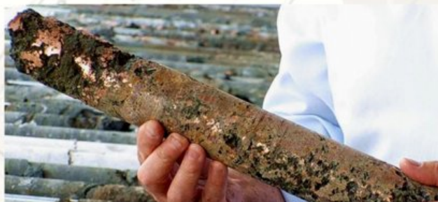
Diamond drill core...solid native copper
