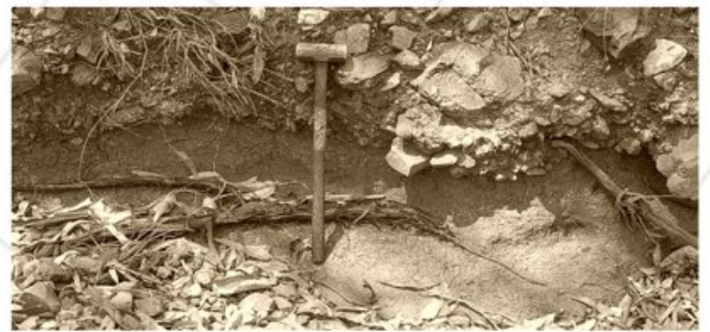
Weathered Dolerite with overlying recent gravel
