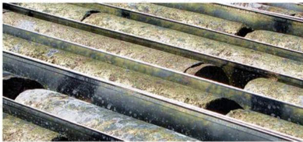
Wide diameter drill core—intense chalcopyrite
