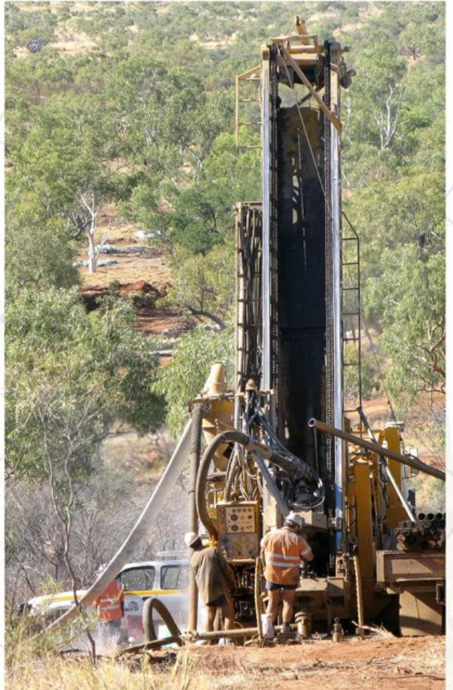
RC rig and crew
