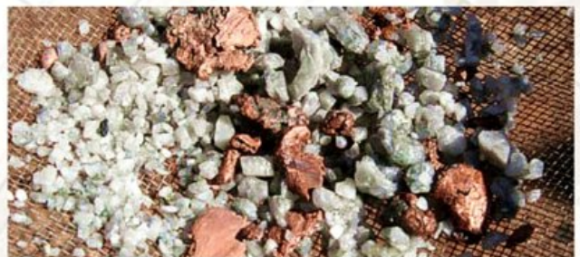
Native copper metal in RC chips
