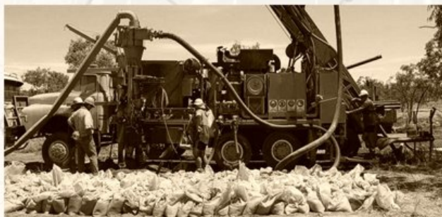
RC drill rig, crew and sample bags
